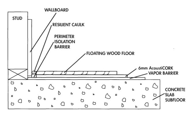
Floating Wood Floors on a Concrete Slab
