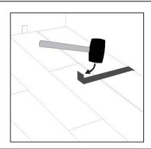
Step 9: Use rubber mallet and pull bar to lock long edges of planks on final row.
