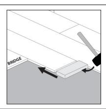
Step 7: Tap end of plank with rubber mallet and tapping block to lock ends of planks together. Remove bridge and continue towards wall until installing the final plank in the row. Be sure to tap on edge if vinyl so as not to damage locking profile.
