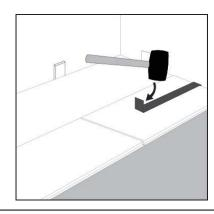
Step 8: Use rubber mallet and pull bar to lock final piece in row. Insert spacer at end of row. Continue installation to final row.
