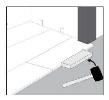
Step 1: Undercut space under door jamb to allow plank to slide freely. Tap long edge with rubber mallet and tapping block to lock long edge.
