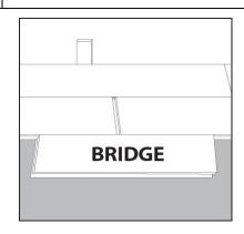
Step 6: Attach a scrap piece of floor to bridge gap between ends of planks.
