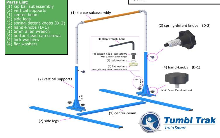
①<u>Attach vertical supports to center-beam</u>
