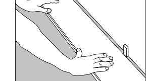
1. After thoroughly cleaning the subfloor, you should begin laying from left to right. Place the floorboard 1/4" from the left wall. Use spacers between the wall and the floorboard.
