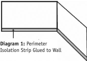
**Diagram 1:** Perimeter Isolation Strip Glued to Wall
