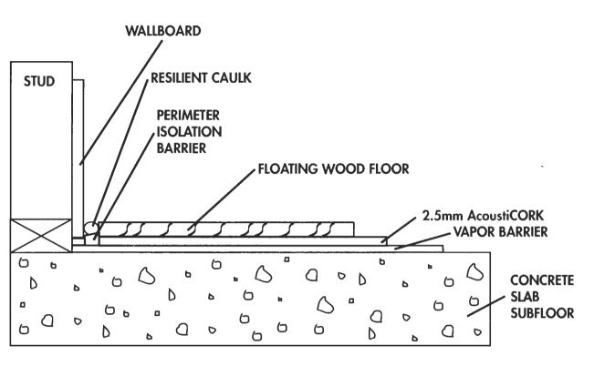
Floating Wood Floors on a Concrete Slab with 2.5mm AcoustiCORK
