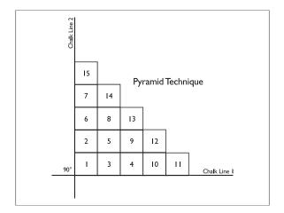
• Always **SLIDE** each module into position from the side to prevent trapped yarn. Set each module by firmly rubbing both joints. Should the StayTac<sup>TM</sup> become contaminated with dust, the back of the module should be wiped with a damp cloth to remove the contamination and restore the effectiveness of the StayTac<sup>TM</sup>
